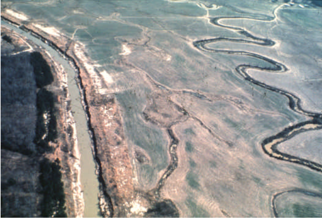
Figure 2.16 Channelized Stream and Abandoned Old Channel
