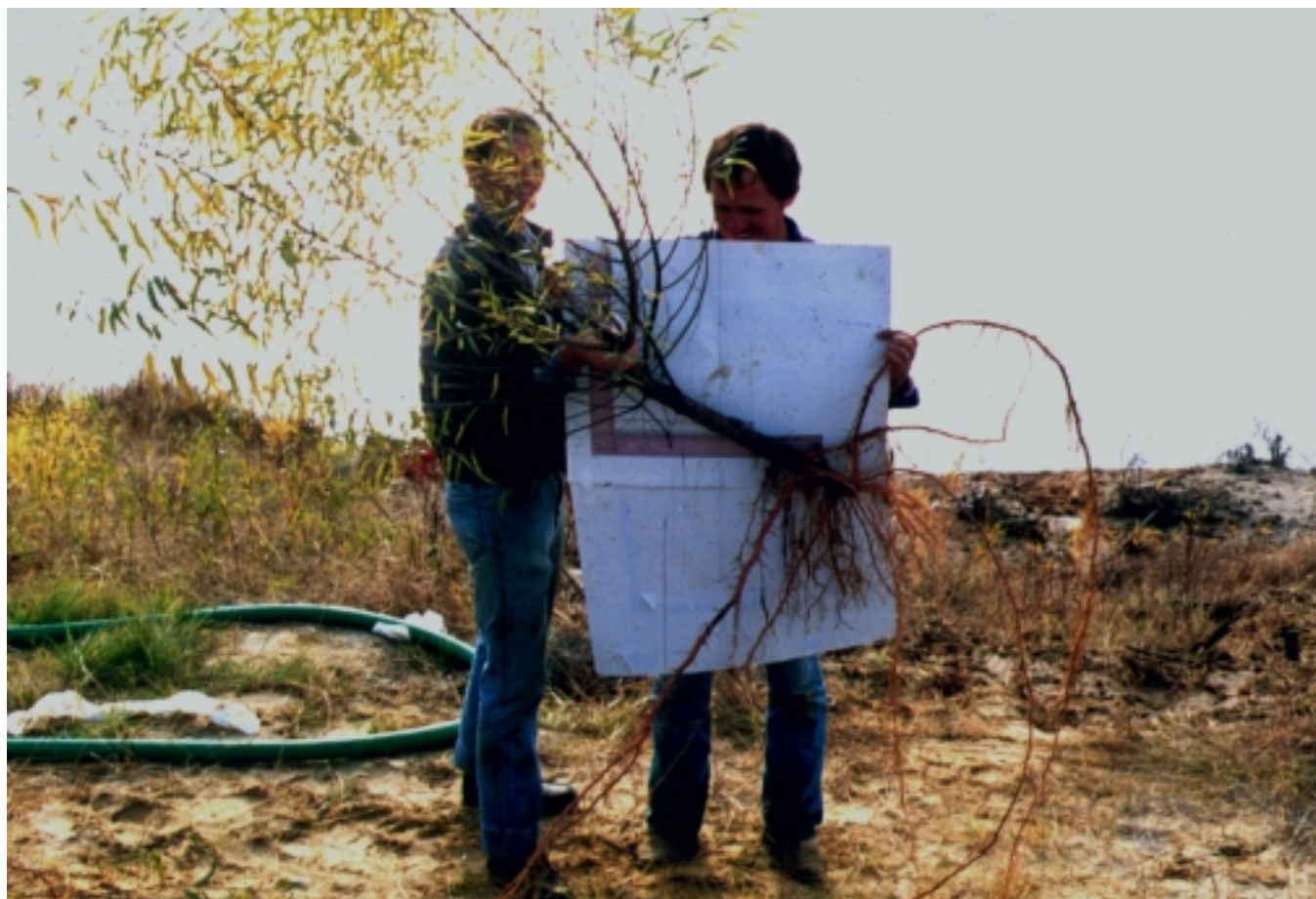
Figure 18–4 Top growth and root development of a 7-month-old live stake (Robbin B. Sotir & Associates photo)
