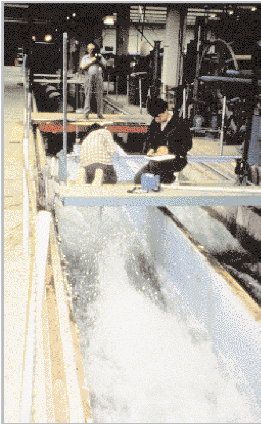
Figure 2. Extensive laboratory flume tests have been conducted to determine the performance limits of RECPs.
