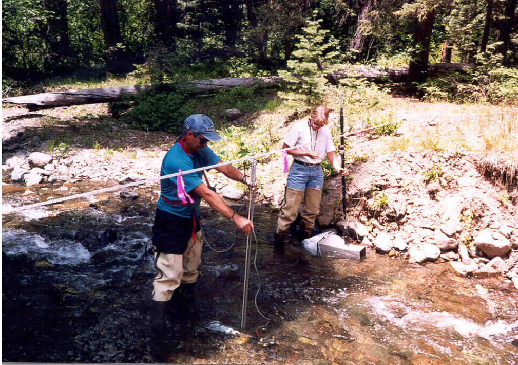
Figure 4.2 Measuring velocity and bedload sediments
