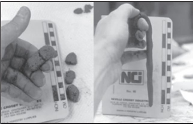
Figure 4. A silty and the clay-like till responded to the ribbon test. The soil on the left is a silty till. Soil on the right is a medium plastic till. The test is a crude measurement of the soil's plasticity (how clay-like the soil is) at a specific moisture content. At appropriate soil moisture content the soil on the right is sufficiently clay-like to support its own weight to a length of approximately 15 cm. Silty or non-plastic soils typically form ribbons two to three cm long. Soils that produce ribbons longer than about three cm are usually somewhat to significantly plastic. The longer the soil ribbon the greater the plasticity and the more clay-like the soil.
