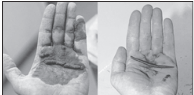
Figure 6. A silty and a clay-like tills response to the toughness test. The soil on the left is a silty or silt-like till. Soil on the right is the clay-like till collected from the sidewall of the largest slope failure shown in figure 1. At appropriate soil moisture content both soils can be rolled out to form thin (approximately 3-mm diameter) soil worms. The soil worm on the left (the silty soil) is very fragile; the soil worm on the right (the medium plastic or clay-like till) is quite durable. Clay-like soils can be rolled out into a soil worm and remolded many times before they refuse to form a coherent soil mass. Ideal granular (non-plastic) soils, such as gravel or sand can not be rolled out into a soil worm. Silty soils can generally be rolled out into weak, fragile, soil worms which quickly lose their ability to form a coherent soil mass with subsequent remolding and rolling.
