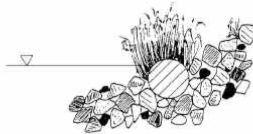
Figure 3. CGR shown at an appropriate elevation to sustain emergent plant growth (from Bestmann GmbH, Wedel, Germany)
