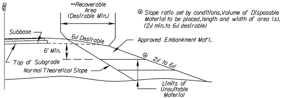
Note: When shoulders are being constructed of commercial material this material shall be extended through the shoulder
