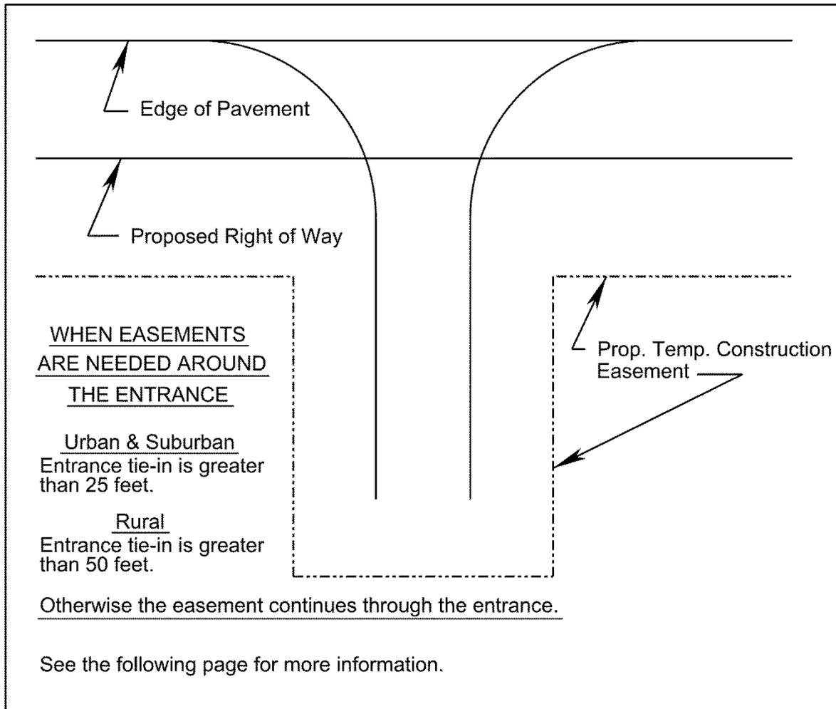
**FIGURE 2E-9 DEPICTING TEMPORARY CONSTRUCTION EASEMENT AROUND ENTRANCES\***
