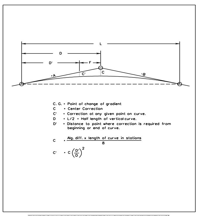
FIGURE C-7-6 PARABOLIC VERTICAL CURVE COMPUTATIONS\*
