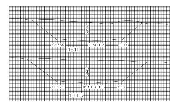
The cut area of station 163+00.02 is 971 square feet, and the area of station 169+50.02 is 769 square feet. To find the average area of the two, we would add the two and divide by two.
