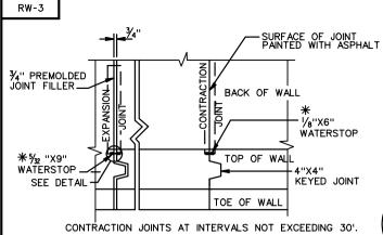
\* WATER STOPS TO BE ELASTOMERIC OR OTHER APPROVED MATERIAL DIMENSIONS SHOWN ARE ABSOLUTE MINIMUM.
