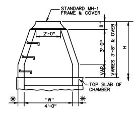
\* WALL THICKNESS TO BE 6" TO A DEPTH OF 10' AND 8" OVER 10'.
