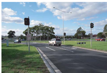
(b) Approach metering signal Melbourne, Victoria, Australia
