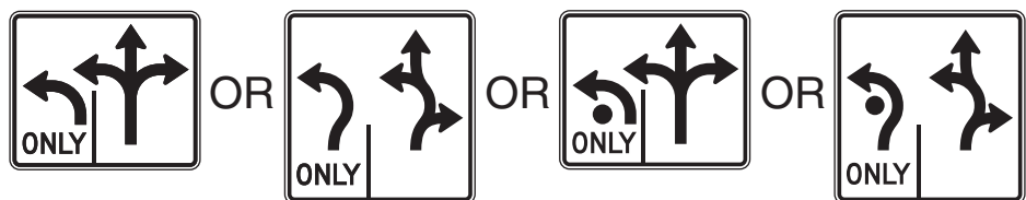
Exhibit 7-16 Intersection Lane-Control Sign Arrow Options for Roundabouts
