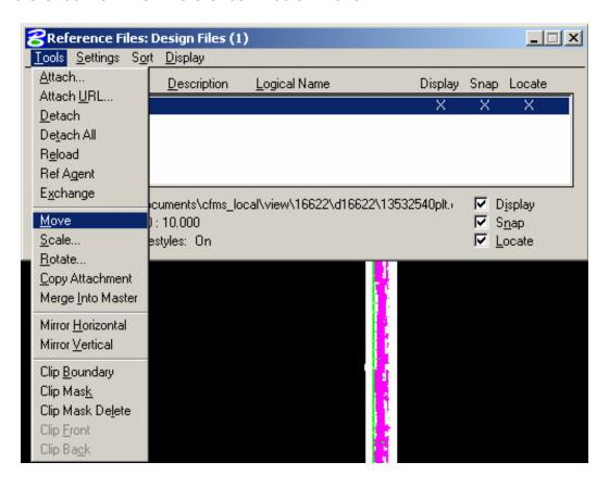
Move the files so they are just above the previous cross section sheets. They should be in the same order they would come in the plan assembly (bottom to top). Fence copy and then detach all reference files.
