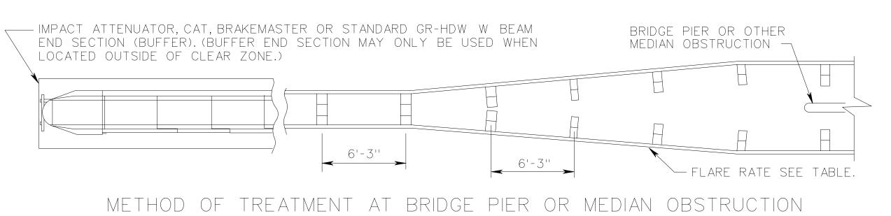
BLOCKED-OUT W BEAM MEDIAN BARRIER
