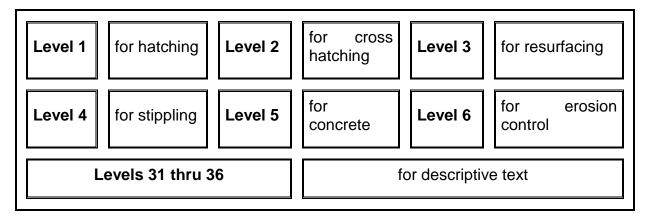
Set proper level. Place shape to be patterned. Set line weight to 1, line style to 0 (LC=0). For resurfacing line style will be 4 (LC=4). See data below for other attributes. The cell for stippling is in dsymgeo.cel, and mdsymg.cel.
