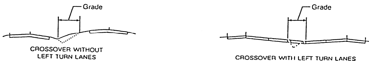
Determination of Grade on a Crossover
