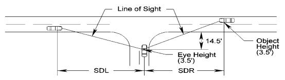
SDR = Sight Distance Right (For a vehicle making a left turn) SDL = Sight Distance Left (For a vehicle making a right or left turn)
