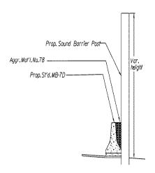
Detail is for Precast Traffic Barrier Service only. If Cast In Place or slip form method is used additional spacing between traffic barrier and sound wall will be required.
