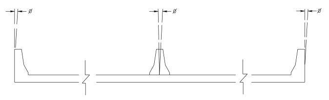
• The barrier should be oriented vertically when the barrier is in front of a retaining wall, as illustrated below:
