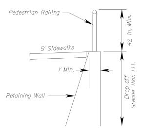
Railing is required when sidewalk is constructed adjacent to a vertical drop-off greater than 1'. However, gripping rail is required <u>only</u> when the grade of the sidewalk is 5% or greater. Contact the Location and Design Standards and Special Design Section for details.
