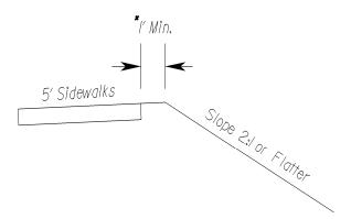
\* No railing is required if a 1' min. graded area is provided at the back of sidewalk when the slope is 2:1 or flatter, unless adjacent to a parallel water hazard 2' deep or other obvious hazard. If a railing is required the graded area behind the sidewalk shall be increased by 1' to accommodate the railing. Contact the Location and Design Standards and Special Design Section for details.
