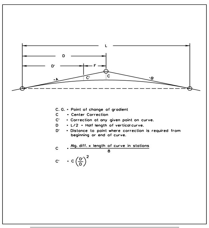
FIGURE C-6-9 PARABOLIC VERTICAL CURVE COMPUTATIONS\*
