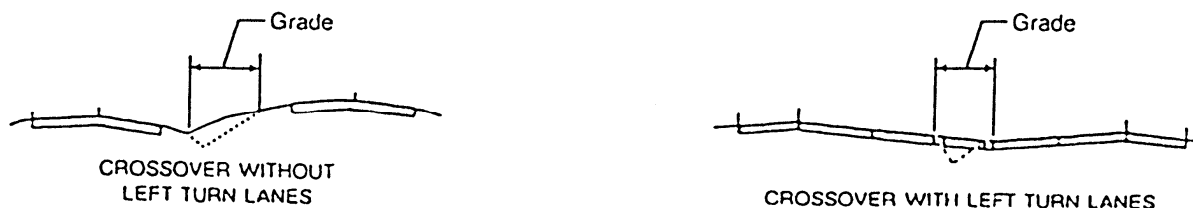
Determination of Grade on a Crossover
