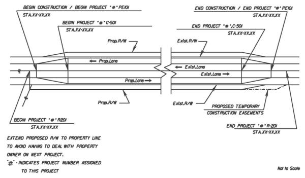
FIGURE 2D - 6 SETTING PROJECT TERMINI\*
