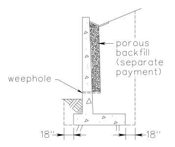
Porous backfill is included in the price bid for Retaining Wall Excavation if only required within an 18" cube for drainage behind the weep hole as required in Section 401.11 of the <u>Road and Bridge Specifications</u>.
