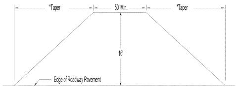
\*Taper Length - See Road Design Manual, Appendix F, Figure 3-1 based on Functional Classification (Rural or Urban) and Design Speed.
