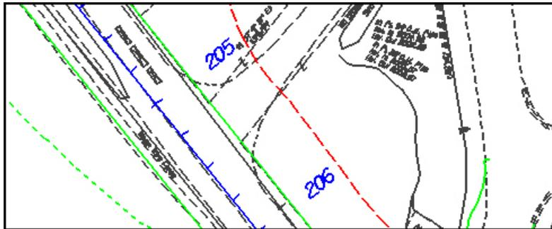
2. Select the Add Drainage Node tool (*Drainage: Component > Node > Add*) and click **OK**.
