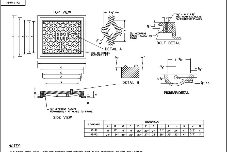
THE COVER SHALL HAVE A NON-SKID SURFACE WITH LETTERS CAST IN THE DEPRESSION ON TOP. THE LETTERS "VDOT ELEC", "VDOT TRAFF", "VDOT COMM" OR "UTILITY" AS APPLICABLE ARE TO BE ONE (1) INCH WIDE AND RAISED!/A" HIGH. COVERS USED FOR JUNCTION BOXES INSTALLED WITHIN MUNICIPALITIES AND NOT MAINTAINED BY VDOT SHALL NOT REQUIRE THE VDOT REFERENCE.
