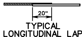
TYPICAL LONGITUDINAL LAP BARS TO BE SECURELY FASTENED TO PREVENT SEPARATION DURING CONCRETE PLACEMENT.
