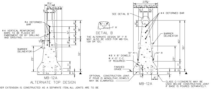
IF BARRIER EXTENSION IS CONSTRUCTED AS A SEPARATE ITEM, ALL JOINTS ARE TO BE CONSTRUCTED AT THE SAME INTERVAL AS CONCRETE BARRIER. ALL JOINTS ARE TO BE ARE #4 AT 24" MAX. SPACING, LENGTH OF DOWELS SHALL BE 20". VERTICAL BARS MAY BE PLACED IN THE CONCRETE OR BONDED INTO DRILLED HOLES IN HARDENED CONCRETE. WHEN HOLES ARE DRILLED NON-SHRINK GROUT SHALL BE USED TO BOND THE BARS IN PLACE.
