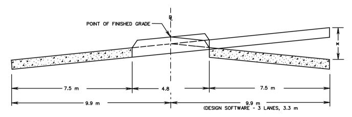
\* THE ELEVATION DIFFERENTIAL BETWEEN NORMAL CROWN AND MAXIMUM SUPERELEVATION, RELATIVE TO THE BASELINE PROFILE.
