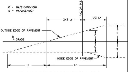
NOTE : ON THE INSIDE OF CURVE THE STANDARD PAVEMENT CROWN (C) SHALL BE HELD UNTIL IT IS EXCEEDED BY THE TABULATED RATE OF SUPERELEVATION (E).
