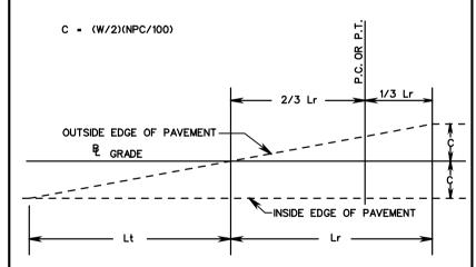
SUPERELEVATED BY AN AMOUNT EQUAL TO THE STANDARD PAVEMENT CROWN
