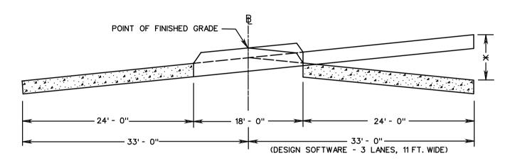
\* THE ELEVATION DIFFERENTIAL BETWEEN NORMAL CROWN AND MAXIMUM SUPERELEVATION, RELATIVE TO THE BASELINE PROFILE.
