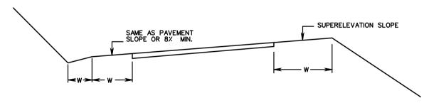
FOR WIDTHS OF SHOULDERS AND DITCHES (W) SEE STANDARDS.
