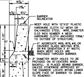
THE ENGINEER. LOCATE WITHIN LOWER SLOPE FACE OF BARRIER TO DRAIN TO ROADWAY. DOWELS AND OPTIONAL CONSTRUCTION
