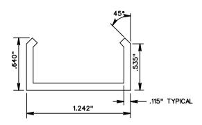
THE MAXIMUM NUMBER OF SPLICES IN A STIFFENER SHALL BE ONE PER STIFFENER LOCATION.
