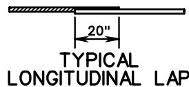
TYPICAL LONGITUDINAL LAP BARS TO BE SECURELY FASTENED TO PREVENT SEPARATION DURING CONCRETE PLACEMENT.
