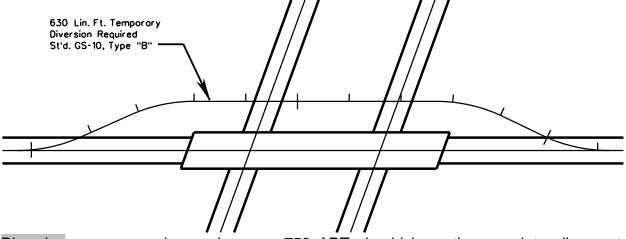
Diversion on crossroads carrying over 750 ADT should have the complete alignment, grades, typical sections, drainage, etc., shown on the plans. Additional temporary construction easement lines should also be shown, if necessary.
