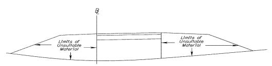
Note: Experience has shown that it is impossible to construct fill with a vertical line clearly separating the good material and the unsuitable material.
