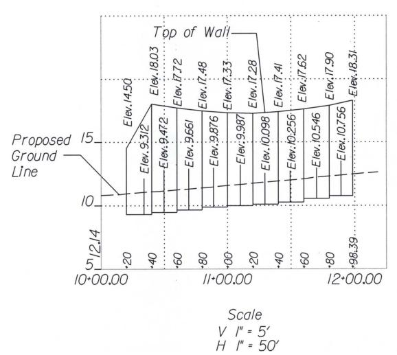
FIGURE 2E-8\* PROFILE FOR PROPOSED RETAINING WALL
