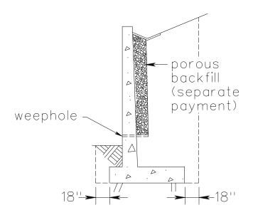
Porous backfill is included in the price bid for Retaining Wall Excavation if only required within an 18" cube for drainage behind the weep hole as required in Section 401.11 of the *Road and Bridge Specifications*.
