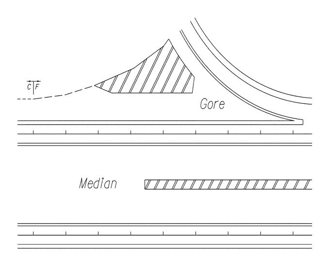
FIGURE 2E-4 TYPICAL METHOD OF SHOWING PLACEMENT OF UNSUITABLE MATERIAL ON PLANS
