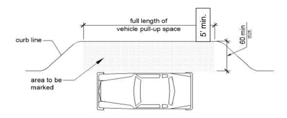
FIGURE C-1-11 PASSENGER LOADING ZONE ACCESS AISLE
