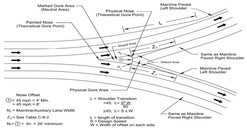
A major fork with neither diverging roadway having priority. The offset is equal for each roadway, and striping or rumble strips are placed upstream from physical nose.
