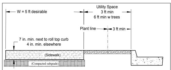
\* If the utility space is paved, construction shall be on compacted subgrade and the thickness shall match that of the sidewalk, however, the area will not be considered part of the minimum width required for sidewalk.
