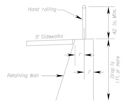
Railing (HR-1 Type II) \*is required when sidewalk is constructed adjacent to a vertical drop-off 1' or greater. However, gripping rail is required only when the grade of the sidewalk is 5% or greater. Contact the Location and Design Standards and Special Design Section for details.
