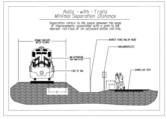
Source: Adapted from the VTrans Pedestrian and Bicycle Facility Planning and Design Manual
