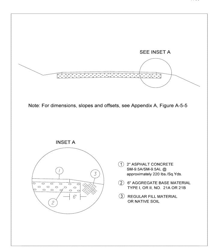
FIGURE A-5-6.1 SHARED USE PATH PAVEMENT STRUCTURE\*
