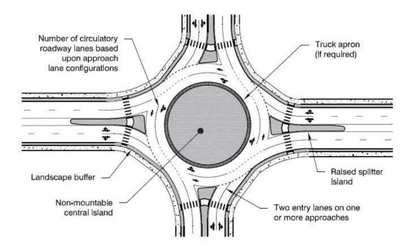
Features of a Typical Multi-Lane Roundabout
