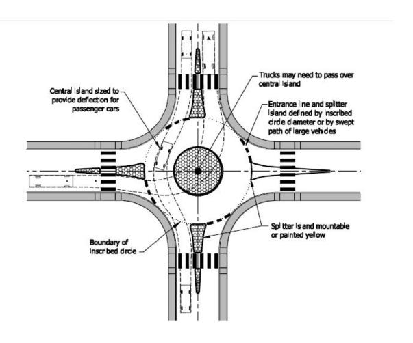
Features of a Typical Mini-Roundabout\*
